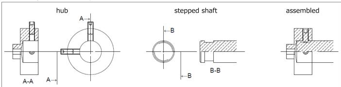
Please note that clearance between the shaft and the hub can cause misalignment with either method.
